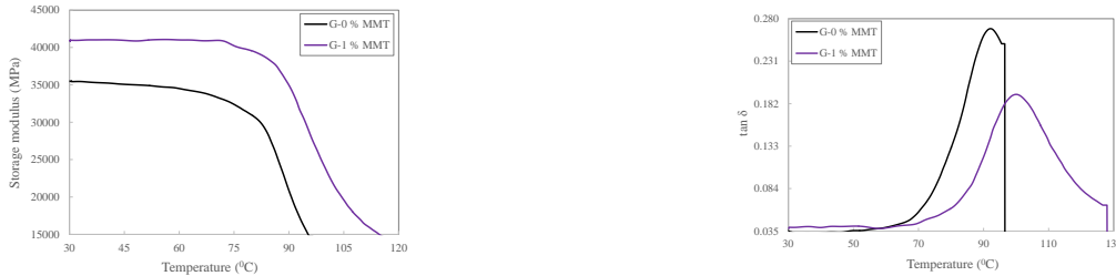
Fig. 5(a) The storage modulus of GFRP composites at 1 Hz (b) The loss factor of GFRP composites at 1 Hz
