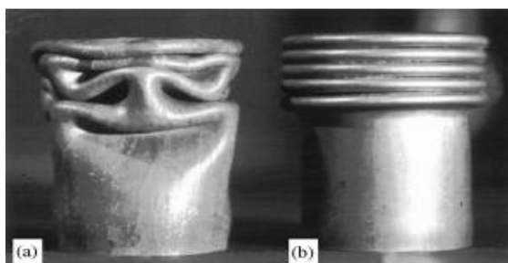
Fig.1. Deformed shape of the 52.6mm diameter steel tube in (a) annealed; and (b) as-received state.
